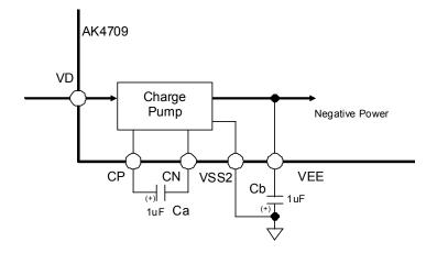
Figure 7. Negative power generate circuit
