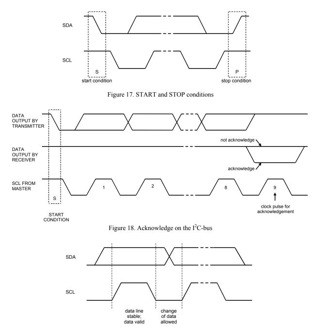
Figure 19. Bit transfer on the I<sup>2</sup>C-bus
